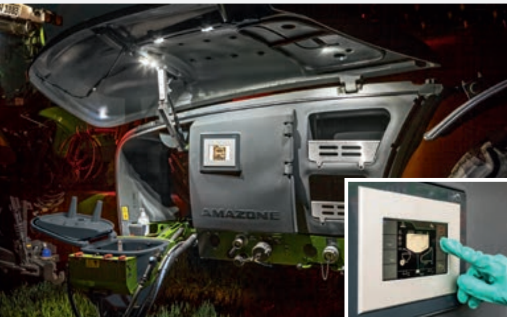
SmartCenter ar LED apgaismojumu un Comfort plus paketi
